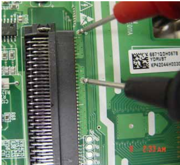
Normal diode value= 0.4 (forward)
