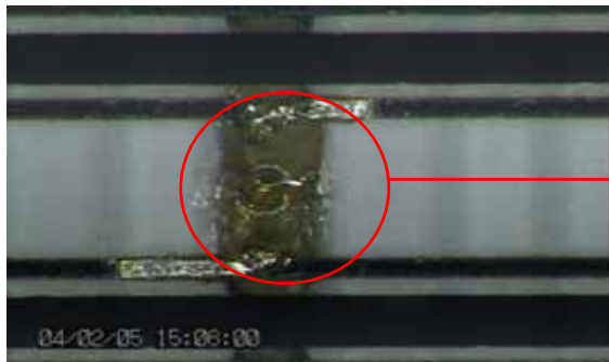
Panel electrode Insulation break down
